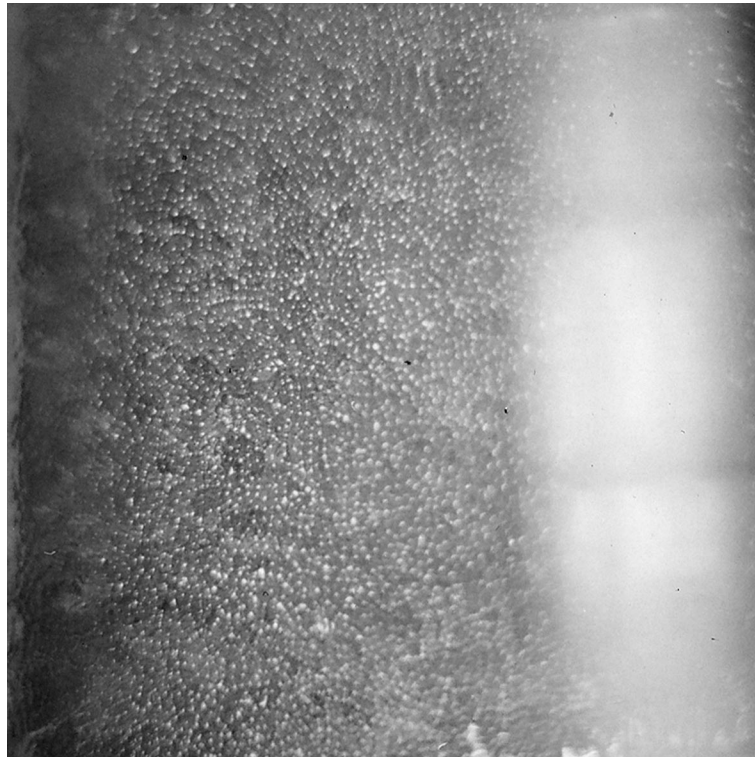
Fig. 11. Photograph of a very coarse melting front like a sharkskin.
